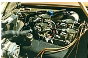
Custom induction system with 4 down draft Rochester two barrel carbs
